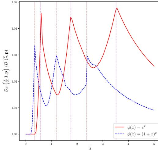
**Fig. 7:** Evolution of the ratio of social costs as a function of the total traffic demand for  $\phi(x) = e^x$  and  $\phi(x) = (1+x)^2$  when there are  $K = 5$  users and  $N = 4$  links, each of a different type. The cost parameters of the links are as follows:  $c_1 = 1$ ,  $c_2 = 2$ ,  $c_3 = 4$  and  $c_4 = 8$ .
