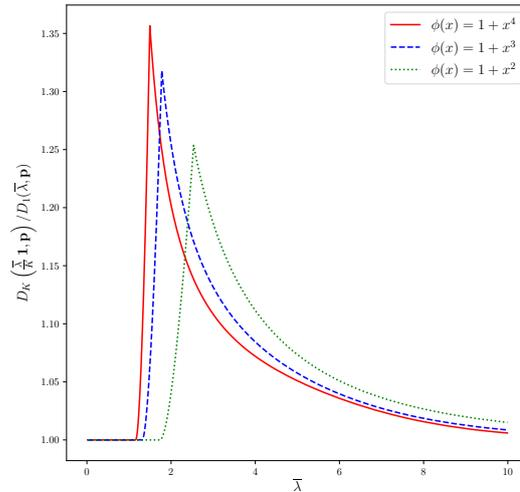
**Fig. 6:** Evolution of the ratio of social costs as  $\bar{\lambda}$  increases for the latency function  $\phi(x) = 1 + x^m$ . In this example, there are  $K = 5$  users, one cheap link with  $c_1 = 1$  and nine expensive links with  $c_2 = 10$ .
