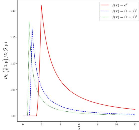
**Fig. 3:** Evolution of the ratio  $D_K\left(\frac{\bar{\lambda}}{K} \mathbf{1}, \mathbf{p}\right) / D_1(\bar{\lambda}, \mathbf{p})$  as  $\bar{\lambda}$  increases for the latency functions  $\phi(x) = e^x$ ,  $\phi(x) = (1+x)^3$  and  $\phi(x) = (1+x)^4$ . The setting is the same as in Figure 2.
